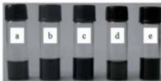
Fig. 10. Dispersion of rGO prepared by \gamma -ray irradiation-based reduction of GO in the DMF. The dispersion of rGO in (a) isopropanol, (b) glycol, (c) DMF, (d) THF, and (e) NMP solvent are shown after two weeks to demonstrate dispersion stability. Reproduced with permission [142].
