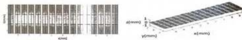
Fig. (1) Design format of linear array transducer (Height=5mm, Width=0.25mm, Kerf=0.02mm)
